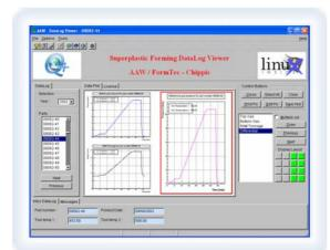
DlgView is another data visualization application used to show data coming from the superplastic forming process. This process uses air pressure to form metal sheets (special aluminium alloys) into specific complicated shapes (e.g. car body parts).
