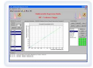
The multivariable regression (MVR) calculation is an empirical correction procedure to minimise, in a multicomponent matrix, the influence of interfering elements on an analyte.
